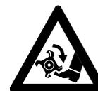
**Risk of injury** from contact with rotating blades. The blades begin to rotate as soon as the engine is started in the "Start" position. Always
